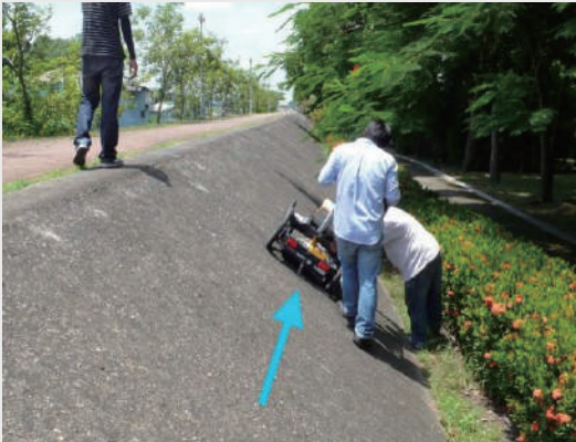
Ground Penetration Radar
